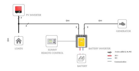
An off-grid system is well suited to rural areas with little or no grid connection but is unlikely to be a viable solution in a well-connected urban area.
