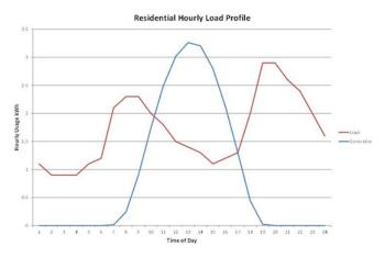
With this example, reducing the size of the PV system by 50% would all but eliminate the surplus but would reduce the useful energy generated by 30%. In the same example there is about 8kWh of surplus energy which could be used to recharge a battery for use in the evenings. The use of a time switch on a washing machine and/or dishwasher can help to maximise the use of generated energy during the sunshine hours.
